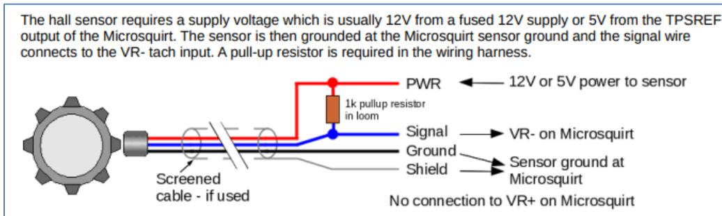
10. We supply the HALL Assy. with a pre-made cable. It must be connected to MicroSquirt (via supplied DEUTSCH 3-pin connector) as follow:
